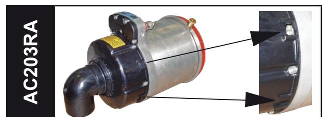
Failure to remove drain plugs will cause build-up of moisture in rear housing and cause aggressive corrosion of rectifier assembly and rapid alternator failure.
